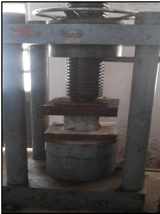
Fig.1- Testing of Cube specimen
