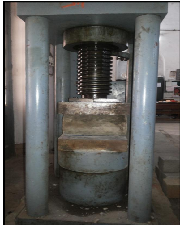
Fig.2 – Testing of Cylinder specimen
